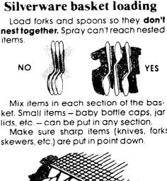
ket. Small items – baby bottle caps, jar lids, etc. - can be put in any section. Make sure sharp items (knives, forks, skewers, etc.) are put in point down.
